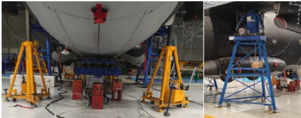
Figure 8 – GRT soft suspending system setup
