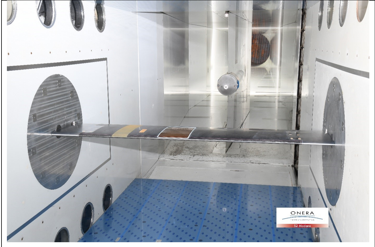
Figure 1: STUNT model mounted in the S2MA ONERA wind tunnel
