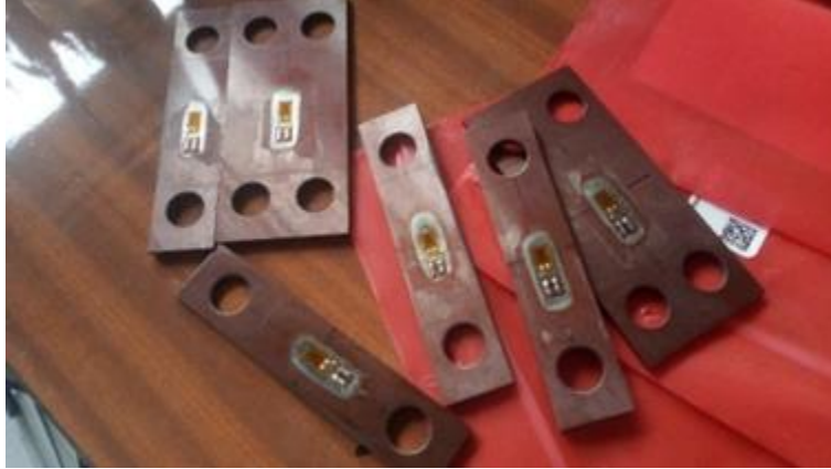
Figure 21: Strain gauges for measurement of pitch and yaw deformation angles.
