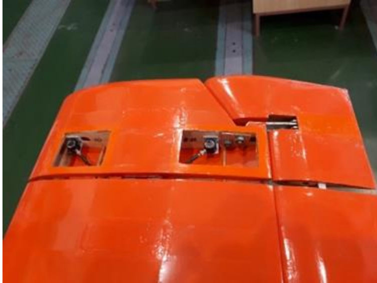
Figure 19: Wing accelerometers installation (wingtip section).
