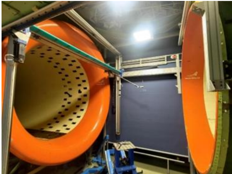
Figure 22: Installation system for flow field sensors.
