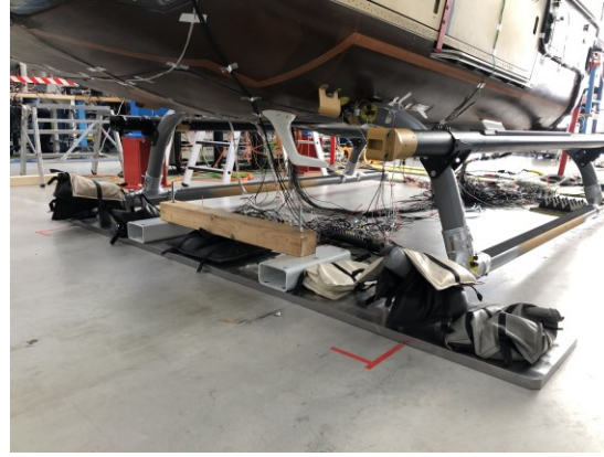
Figure 8 Ground resonance for slope landing
