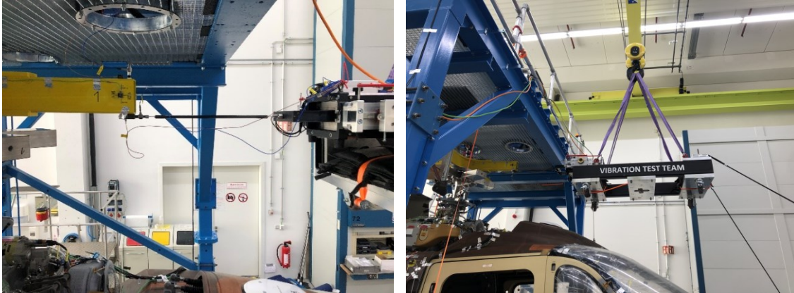
Figure 14: Excitation at main rotor in Tx direction with shaker and reaction mass hung from hall crane
