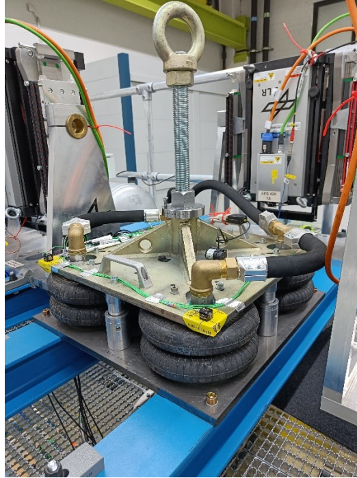
Figure 6: Mechanical part of pneumatic suspension system
