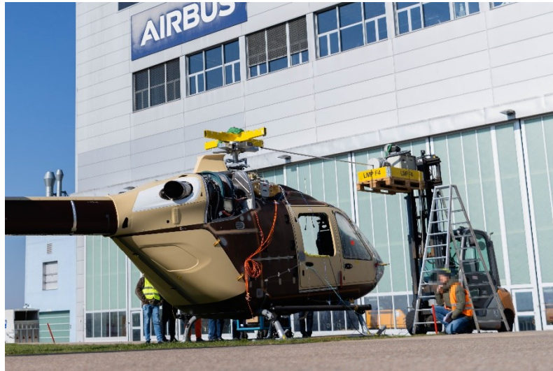
Figure 24: Ground Resonance Test of Helicopter Demonstrator
