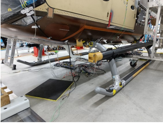
Figure 7 Ground resonance test with skid on concrete
