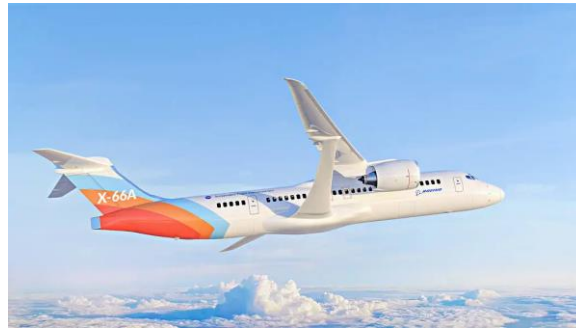
Strut- and truss-braced wings
