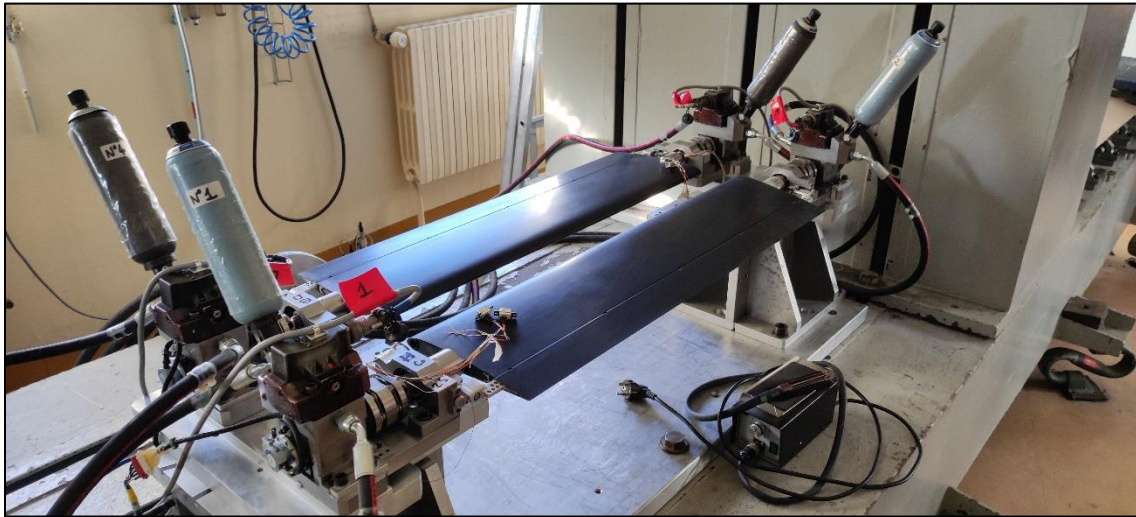
Figure 11 : Laboratory characterisation of the movable flapped vanes gust generator
