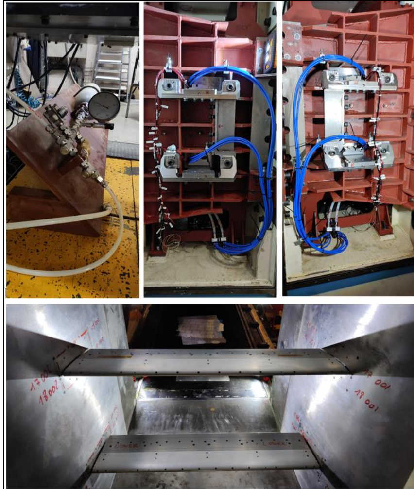
Figure 18 : Fixed vanes gust generator installed in the final part of the wind tunnel convergent section (bottom) – Mounting part and pneumatic supply line (top)
