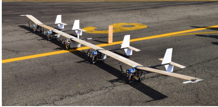
Figure 1: X-HALE prototype with a 6-meter wingspan from ITA/LNCA. Source: LNCA Internal Archive
