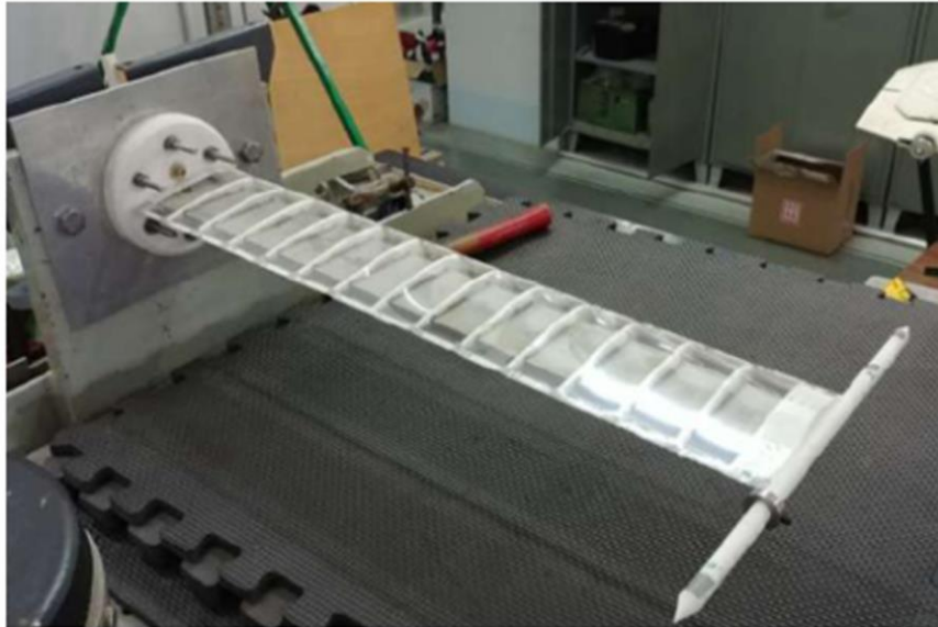
Figure 4 Pre-pazy wing model test setup
