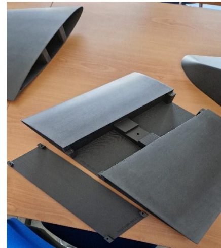
Figure 3: a 3D printed aerodynamic sector
