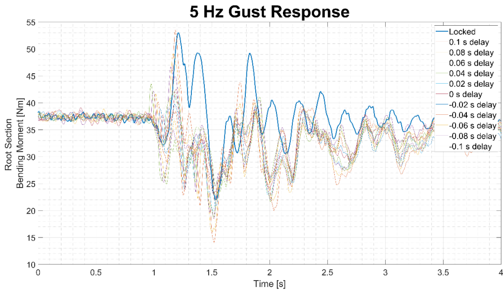
Figure 19: root bending moment time history. Comparison between the locked wing tip conditions and different time intervals between the gust and the unlocking of the wing tip
