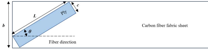
Figure 2. Ply angle and section length, where, the fiber fabric width is b , the ply lamina width is c and each lamina's length is L .
