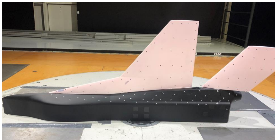
Figure 8: Aeroelastic wind tunnel model on the turn table of the Wind Tunnel at the Technical University of Munich.
