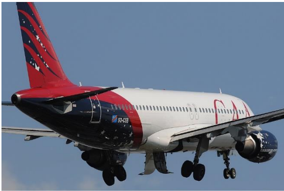
Figure 1: Airbus A320-212 with main landing gear doors open. Nose and main landing gears are in transit [13].
