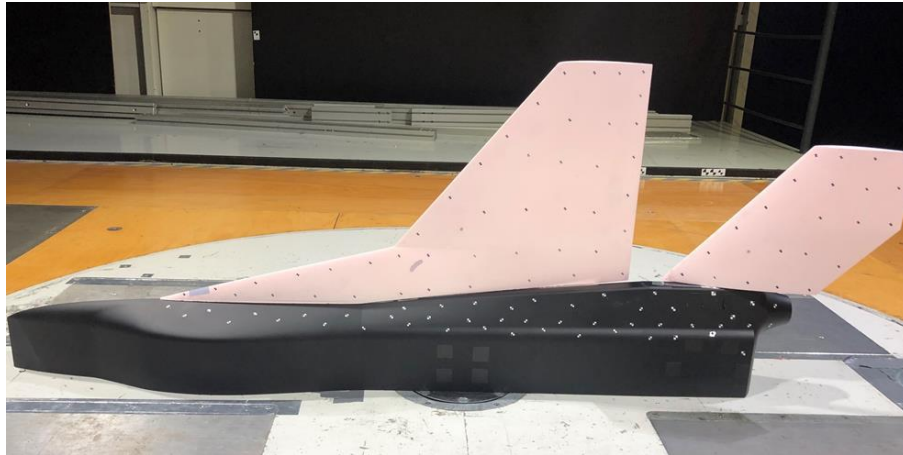
Figure 6: aeroelastic wind tunnel model at the Technical University of Munich
