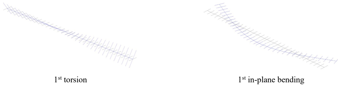
Figure 7. Primary elastic modal shapes of single aircraft
