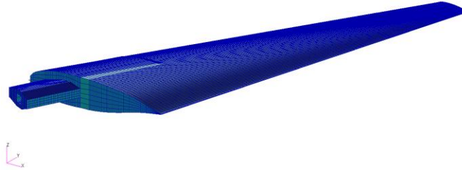
Figure 15: The finite element model of the wing with the support beam.
