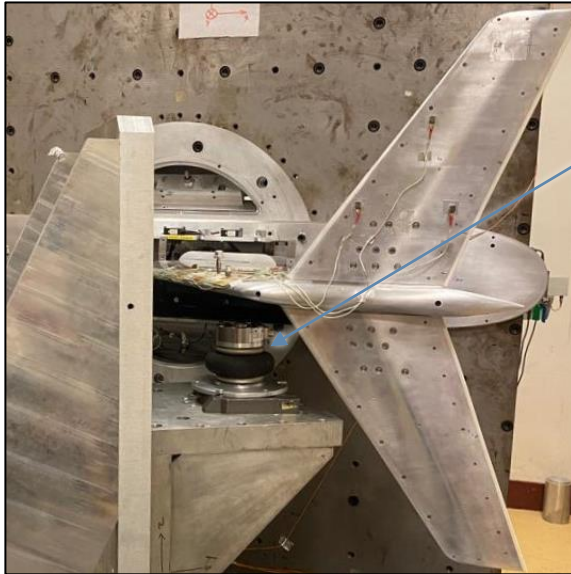
Figure 3-6 Static tests on the horizontal stabilizer
