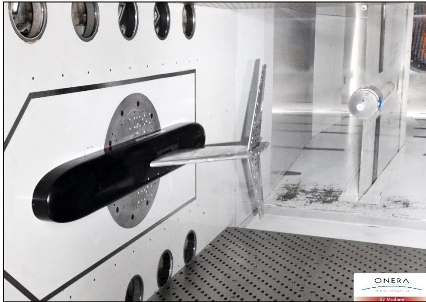
Figure 4-1 T-tail model ( T-2^\circ ) inside the S2MA transonic wind tunnel
