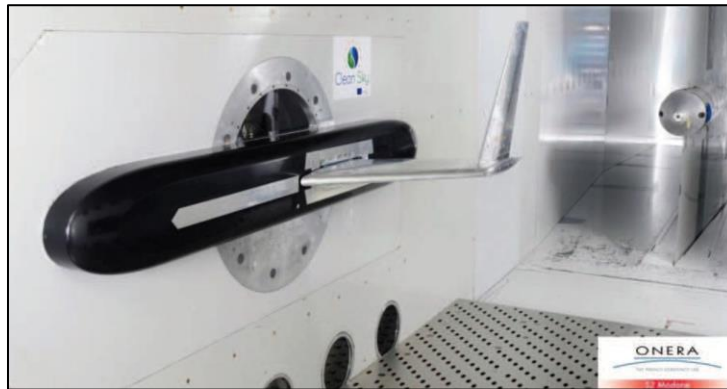
Figure 1-1 Photo of Clean Sky 1 U-tail flutter test
