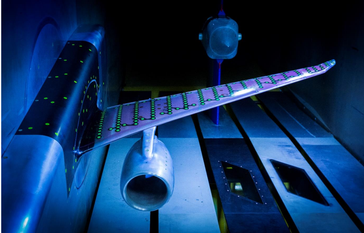
Figure 1: Transport aircraft wing model mounted in DNW-HST.
