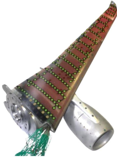
Figure 6: Assembled model outside the wind tunnel section (left) [1].
