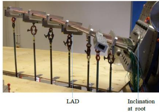
Figure 7: Load and deflection test (LAD is the load application device) [2].
