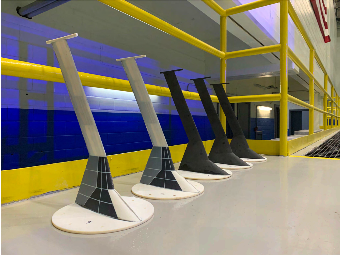
Figure 6: Several aeroelastic models prior to wind tunnel testing, composed of (left two) Polyjet and (right three) HT23
