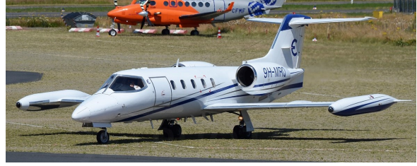
Figure 2: Image of a Learjet 35, featuring wingtip fuel tanks. 2
