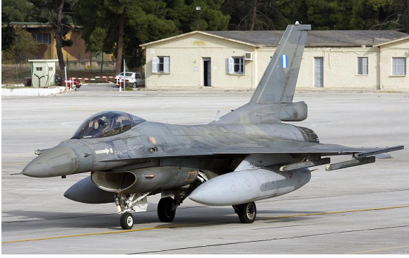
Figure 1: Image of an F-16C Fighting Falcon, with wing mounted drop tanks. 1
