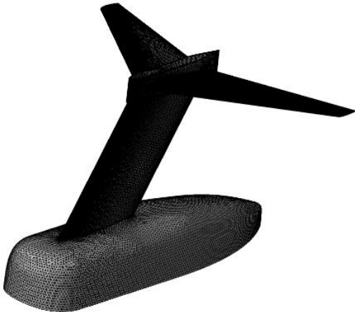
Figure 3 - Surface mesh for CFD analysis
